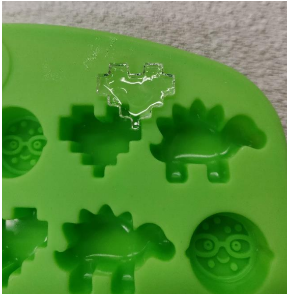
Figure 1: Silicone mold used to shape the hydrogel while curing with UV light.
